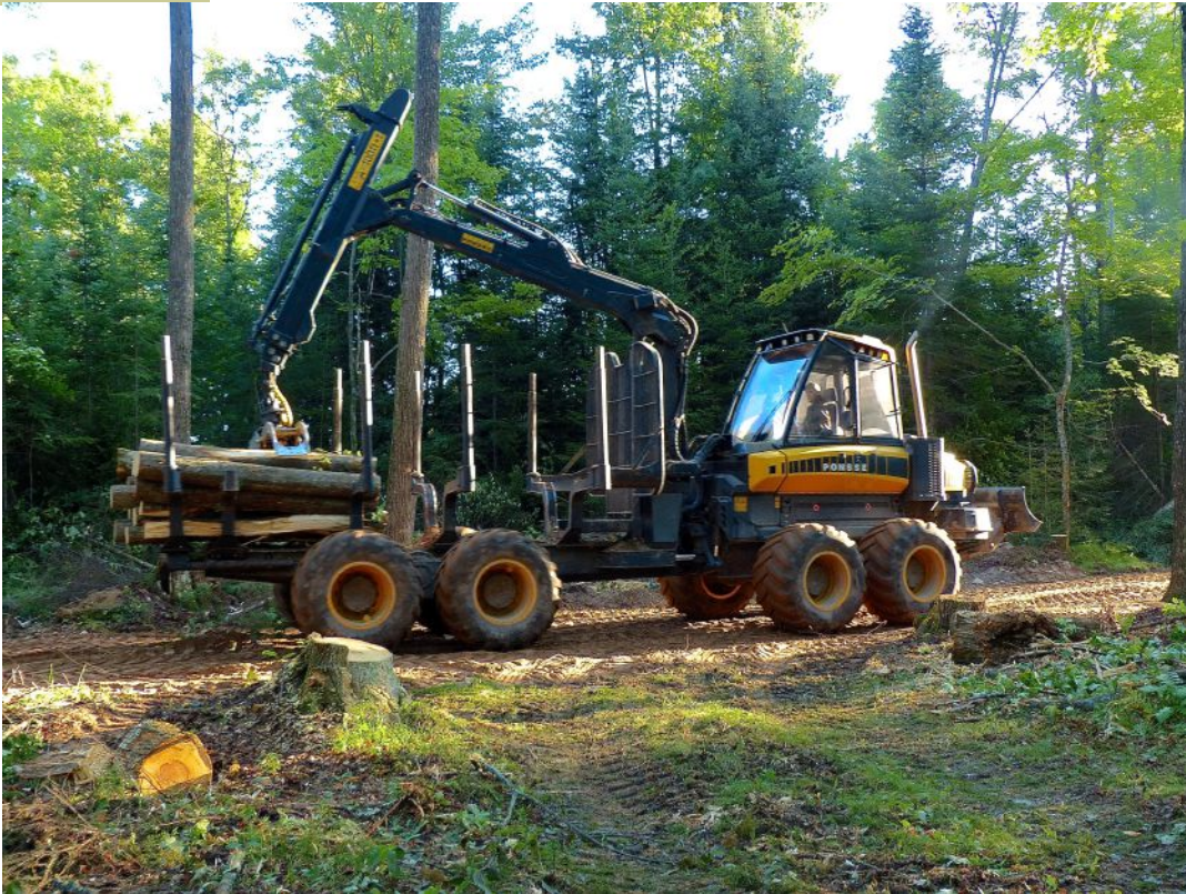
A double bunk forwarder working on an Enterprise Forest Products job. © Schmitt Photography
